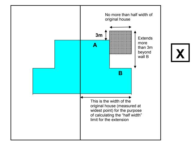
In other cases, an extension may comprise both elements of a rear and side extension. Examples could include:
