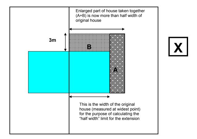
In the example above, if the side extension  $\bf A$  was built first, it would meet the requirement for being no more than half of the width of the original house. However, the later addition of the rear extension  $\bf B$  would mean that the total width of  $\bf A$  +  $\bf B$  at the widest point would be more than half the width of the house. The rear extension would therefore require an application for planning permission.
