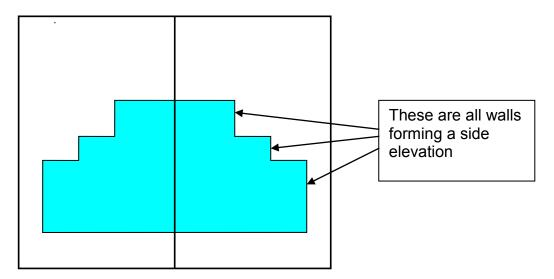
Where an extension is beyond any side wall, the restrictions in (j) will apply. Any extension can only be a single storey, must be less than 4 metres in height and can only be half the width of the original house. The width of the original house should be calculated at its widest point.
