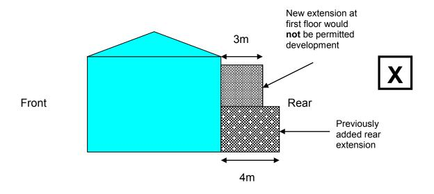
In addition, where the extension or enlarged part of the house has more than one storey, it must be a minimum of 7 metres away from any boundary of its curtilage which is opposite the rear wall of the house being enlarged. For example:
