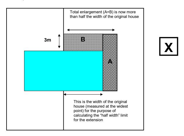
In the example above, if the side extension  $\bf A$  was built first, it would meet the requirement for being no more than half of the width of the original house. However, the later addition of the rear extension  $\bf B$  would mean that the total width of  $\bf A$  +  $\bf B$  at the widest point would be more than half the width of the house. The rear extension would therefore require an application for planning permission.
