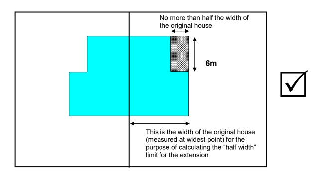
In the following example, although the extension is less than half the width of the original house and extends beyond the rear wall at 'A' by only 3 metres, it extends beyond the rear wall 'B' by more than 6 metres (or 3 metres on article 2(3) land or sites of special scientific interest). It would therefore not be permitted development and will require an application for planning permission.
