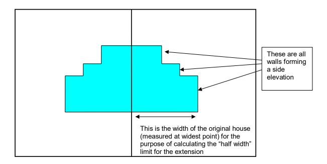
Where an extension is beyond any side wall, the restrictions in (j) will apply. Any extension can only be a single storey, must be less than 4 metres in height and can
