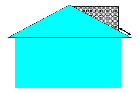
Minimum of 0.2m from eaves to edge of the enlargement to be measured along the roof slope from the edge of the enlargement to the outer edge of the eaves. The enlargement cannot overhang the outer face of the wall of the original house.
