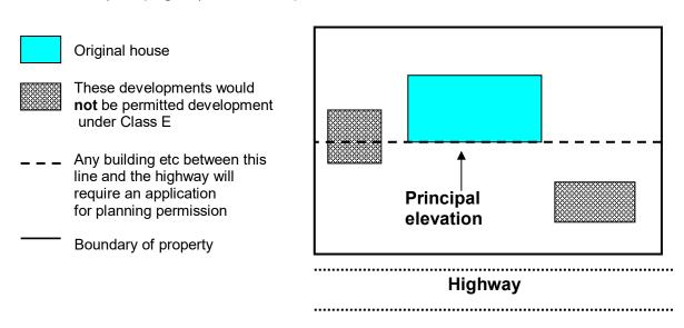
Where the principal elevation comprises more than one wall facing in the same direction, all such walls will form part of the principal elevation and the line for determining what constitutes 'extends beyond a wall' will follow these walls:
